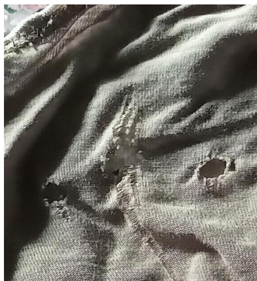
Fig6: Hole on Single Jersey Knitted Fabric
