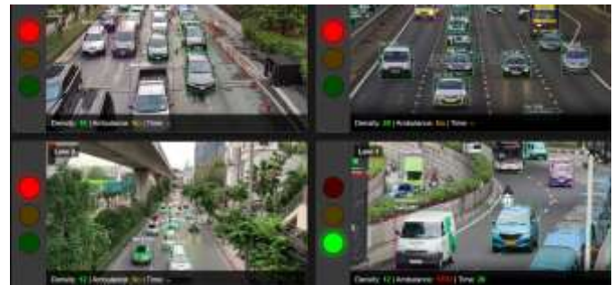
Fig. 3. Live Traffic Monitoring Dashboard showing real-time vehicle detection, signal status, and lane-wise density across multiple lanes
