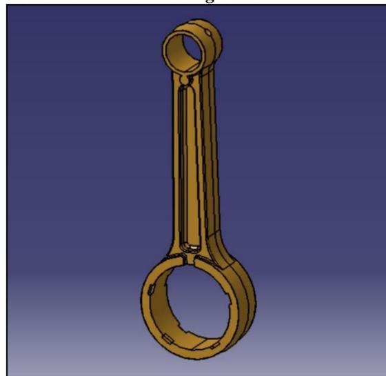
Fig.3.3. 3D model of connecting rod
