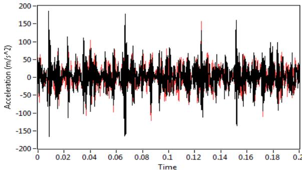
Fig.5a) Time domain signal for defective bearing at 1800 rpm (Inner race line defect)
