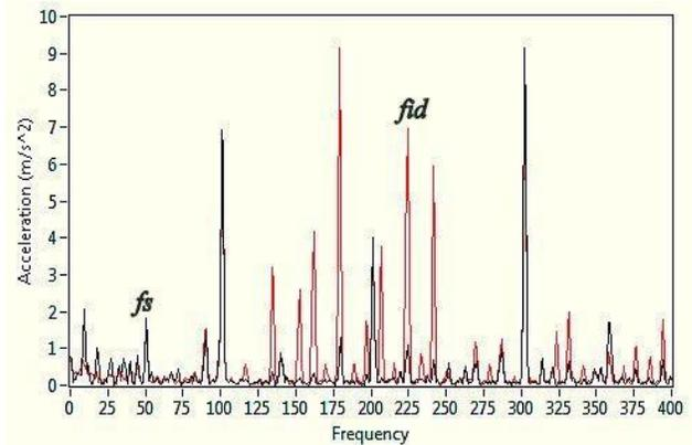
Fig.6b) Spectrum of defective bearing at 2400 rpm (Inner race line defect)
