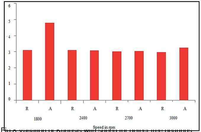
Fig. 8 Variation of Kurtosis with speed for defect free bearings
