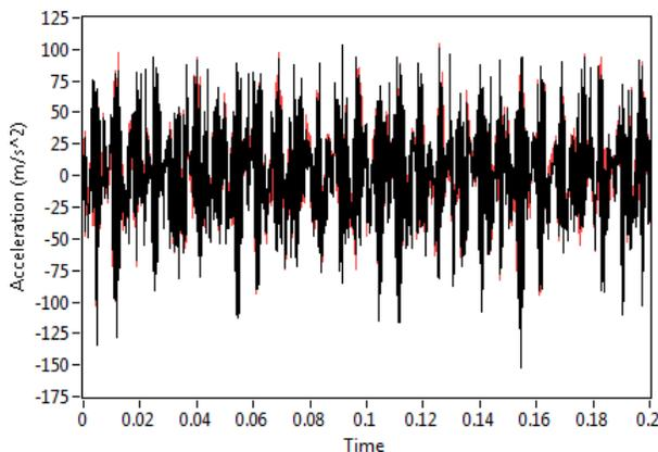
Fig. 3a) Time domain signal for defective bearing at 1800 rpm (Outer race & Ball) in radial and axial direction
