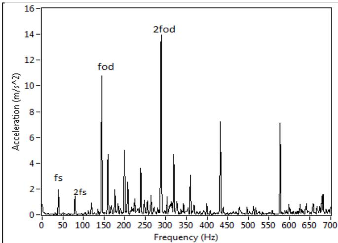
Fig. 7 Spectrum of defective bearing with defect on outer race at 2400 rpm
