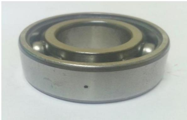
Fig.3 Defective Bearing with 1mm defect on outer race
