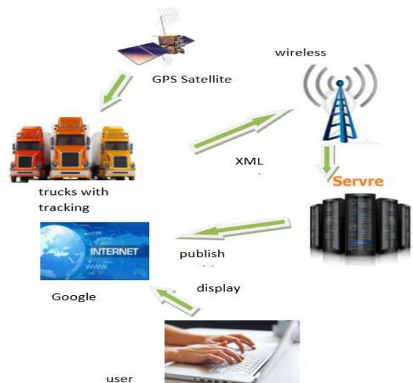
Figure 8: The Trucks Tracking System Overview
