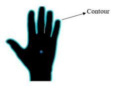
**Convex Hull and Defects:**Convex hull points most likely to be on the fingers as they are the extremities and hence this fact can be used to detect no offingers. We are finding the deepest point of deviation on the contour.
