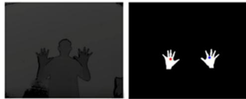
**Contour Extraction:** Contour extraction is performed using Open CV's inbuilt edge extraction function. It uses a canny filter. You can tweak parameters to get better edge detection.
