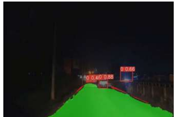
Fig 2: Lane detection using CNN
