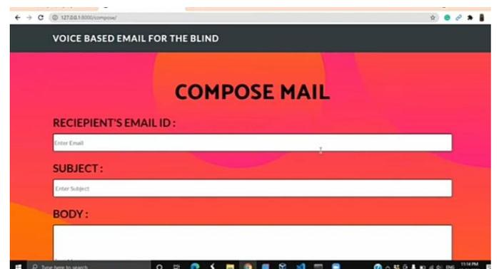
Required information of the receiver's mail, subject, body details are filled through voice and the details are updated. Finally the mail is sent to the receiver. Hence the complete emailing process is done only by voice such as logging in to the system, selecting the option such as composing the mail and the sending the mail to the desired user.
