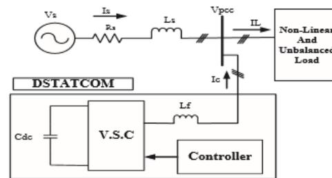
Proposed system introduces a new concept of DTATCOM that Use conventional FACTS and D-FACTS devices. The DPFC gives the possibility of control all system parameters, such as line impedance and power angle, mitigate sag, swell and Harmonics. At the same time, it provides higher reliability and lower cost.
