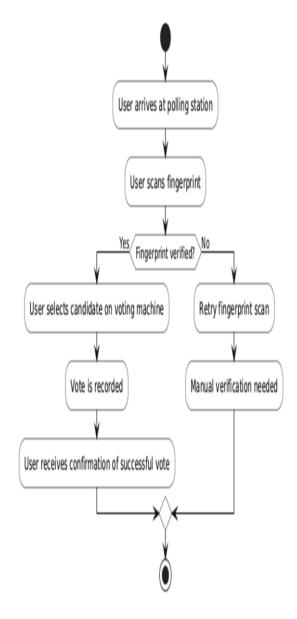
FIG.1. FLOWCHART FOR VOYING SYSTEM USING FINGERPRINT
