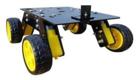
The chassis provides structural support, housing the various components such as the motors, microcontroller, and sensors. It is designed to be lightweight and durable, allowing the robot to move freely across different floor types. The wheels ensure smooth movement, with their design allowing the robot to traverse obstacles or rough surfaces while maintaining stability
