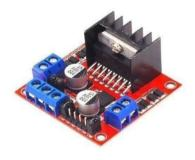
The motors provide the necessary movement to the robot, driving the wheels. The motor driver acts as an interface between the ESP32 and the motors, converting the signals from the microcontroller into physical motion. The driver controls the speed and direction of the motors, enabling the robot to move forward, backward, or turn based on the software's commands. This allows for precise navigation during cleaning operations.
