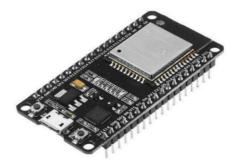
The ESP32 microcontroller is the brain of the robot. It handles all the logic for controlling the robot's movement and decision-making. It processes inputs from the ultrasonic sensors to detect obstacles and also sends control signals to the motors through the motor driver. With its Wi-Fi capability, it allows for remote control and monitoring of the robot, making it adaptable to different environments.
