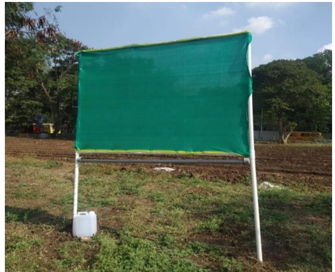
Figure 1. Picture showing the actual fog collector used in the field study
