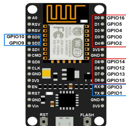
Fig 6. NodeMCU DevKit GPIOs
