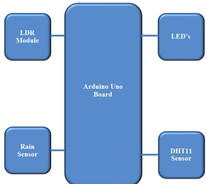
The weather adaptive light intensity controller functions by continuously monitoring real-time environmental conditions using DHT11 (temperature & humidity) and a rain sensor. The system is powered by an Arduino Uno, which processes sensor data and adjusts the bulb's brightness accordingly. The ESP8266 WiFi module enables wireless monitoring and control via an IoT platform.
