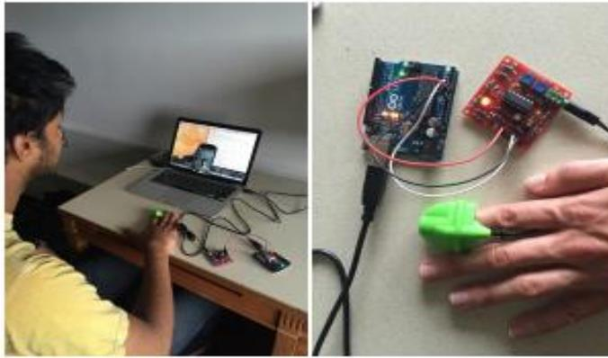
Figure 2. Experimental setup. One-minute videos of a subject's face were captured with a Samsung camera, and a reference PPG signal was recorded using the Easy Pulse fingertip PPG sensor and an Arduino Uno.
