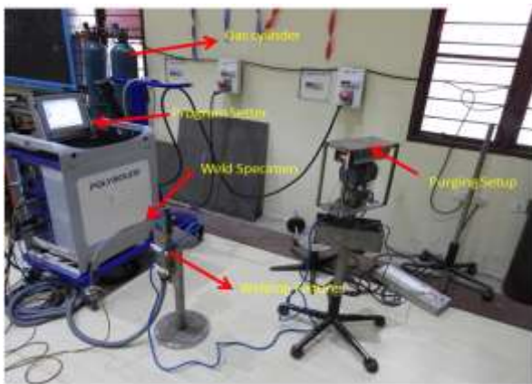
Figure 1: Autogenous weld setup
