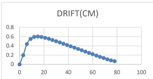
**Fig7 Graph between Height vs. Storey Drift**
