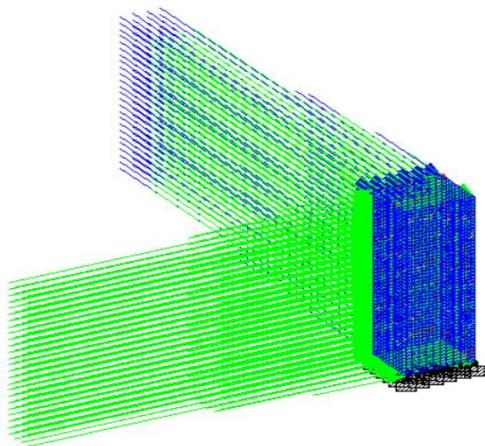
**Fig3 Wind load on structure**
