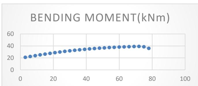
**Fig9 Graph between Storey vs. Bending Moment**
