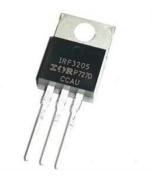
For this project, we used the MOSFET model IRF 3205. A high current N-Channel MOSFET with a switching capacity of up to 110A and 55V, the IRF3205. The MOSFET's unique selling point is its ultra-low on resistance of just  $8.0m\Omega$ , which makes it ideal for switching circuits like inverters and DC-DC converters.
