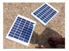
A solar panel is an assembly of photovoltaic solar cells installed in a (often rectangular) frame. It is sometimes referred to as a photovoltaic (PV) module or PV panel. Sunlight is used by solar panels to collect radiant energy, which is then transformed into direct current (DC) power. It is a 10W, 12V monocrystalline solar panel.
