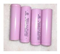
An apparatus that stores chemical energy and transforms it into electrical energy is a battery. Electrons move from one substance (electrode) to another through an external circuit during chemical reactions in batteries. An electric current can be created by the flow of electrons and employed to perform tasks. For this project, we are using 4 lithium-ion batteries with a rating of 3.7v each.
