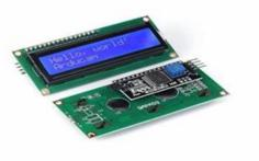
The 16x2 LCD screen, illuminated with yellow and blue backlight, is a versatile component for Arduinobased systems. It is easy to interface with microcontrollers that act as a powerful printing device. The screen can display plain text or numerical information that can be obtained from various sensors, such as temperature or pressure sensors. It can also report the number of Arduino execution cycles and provide realtime insight into system performance.
