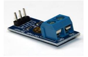
This sensor is used to monitor, calculate and determine the supply voltage. This sensor can determine the AC or DC voltage level. The input of this sensor can be voltage, while the output can be switches, analog voltage signal, current signal, audio signal, etc.
