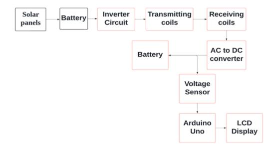
Fig. No. 1- Block diagram of the project. Solar panels produce energy, stored in a battery. Through inverter circuits, it's wirelessly transmitted, converted to DC, processed by an Arduino Uno, and displayed on an LCD.
