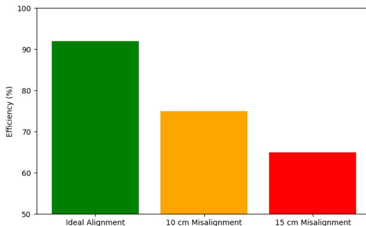
Figure. 3 Power Transfer Efficiency vs. Coil Misalignment
