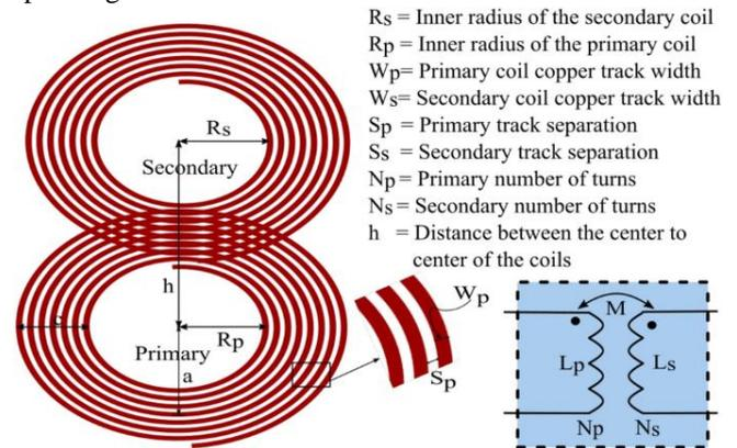
**Figure. 2** Optimization of Circular Coil Design for Wireless Power Transfer System
