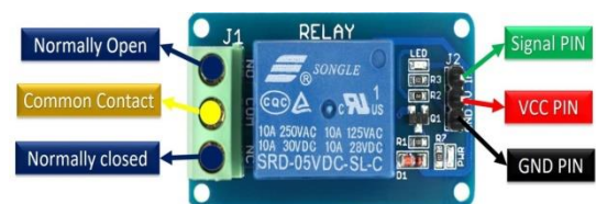
Fig 4.5 5V Relay Module Pin Configuration
