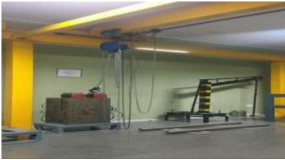
Fig.2. overhead crane installed for the mould maintenance.
