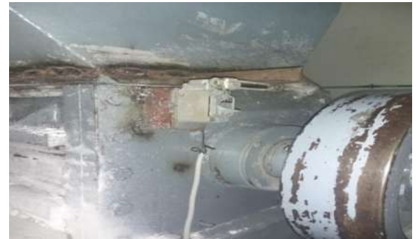
Fig.5. Limit Switch Installed
