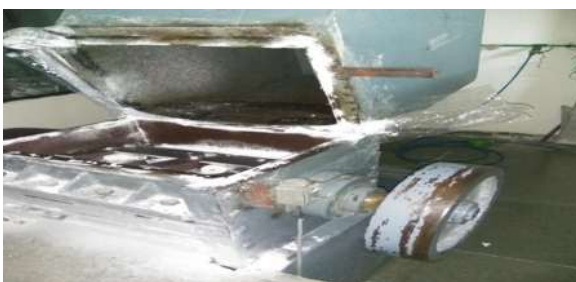
Fig.4. Open gate of grinding machine, inside the machine the sharp blades are there which can cause serious injury.
