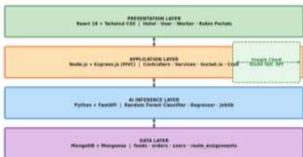
Fig. 2: Four-Layer System Architecture of Zarfo
