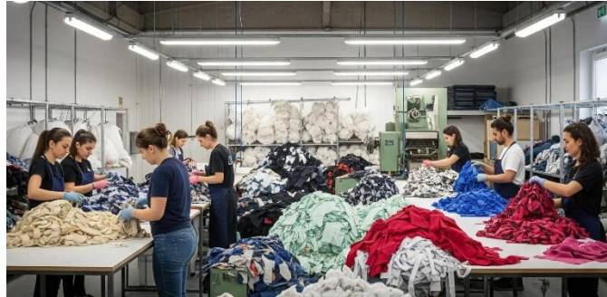
Figure 6. Classification of textile remnants by material, colour, size and texture.
