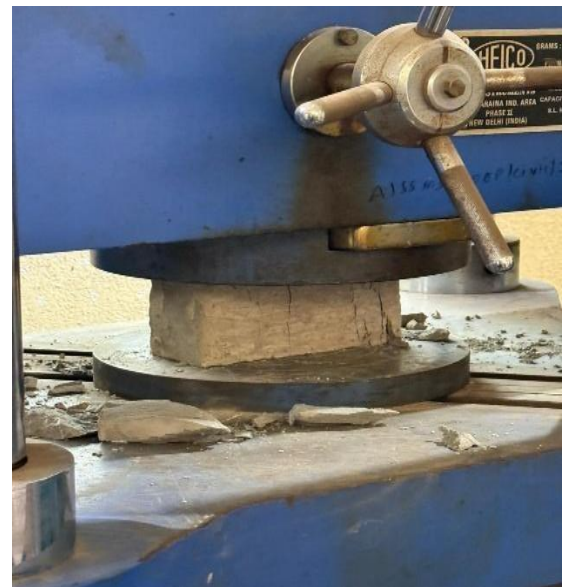
FIG 5 : FAILURE OF BRICK
