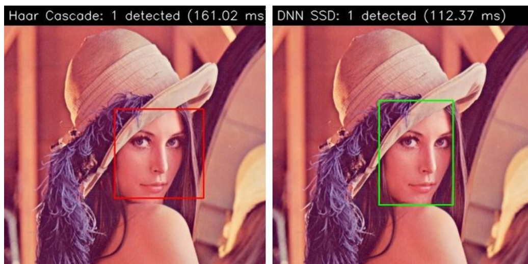
Fig. 1. Lena portrait — Haar cascade (left) vs. DNN SSD (right). Both detectors correctly locate the single face.
