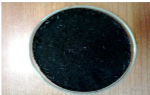
Figure 2 Sugarcane bagasse ash
