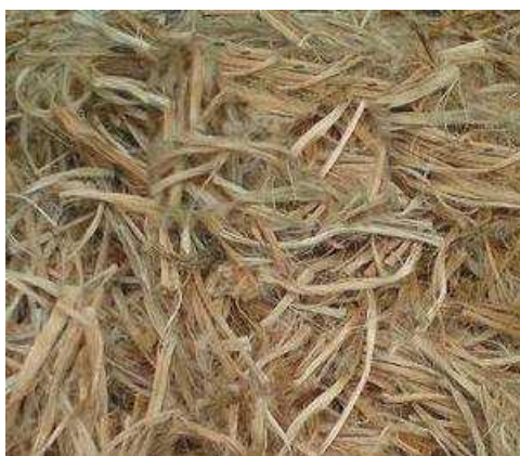
Figure 1 20mm Pieces of jute fibre Admixture
