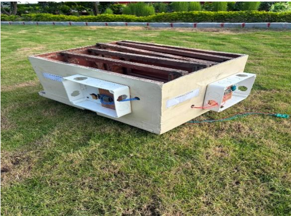
Fig -3: Prototype of the proposed IoT-based smart hive monitoring system.
