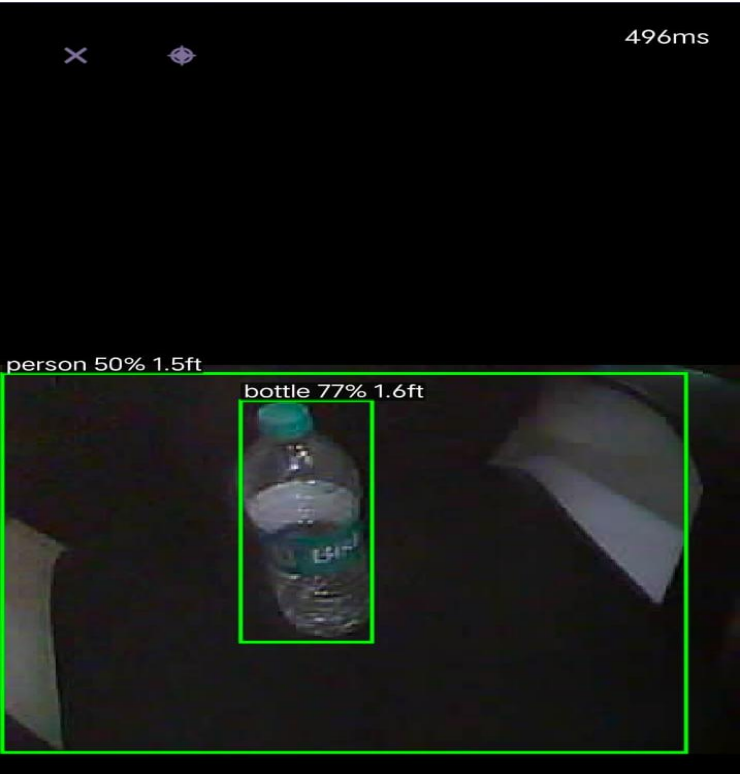
FIG.5. REAL-TIME DETECTION OF A PERSON AND BOTTLE WITH CONFIDENCE SCORES AND ESTIMATED DISTANCES.
