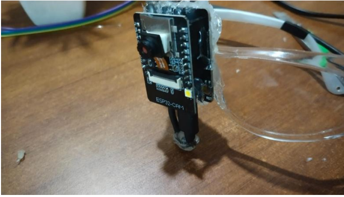
FIG. 3. PROTOTYPE OF THE AI-BASED SMART GLASSES WITH ESP32-CAM MODULE.
