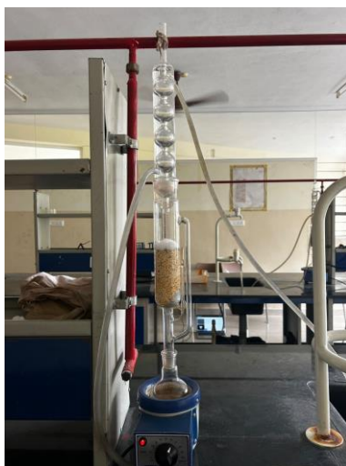
Fig. 2: Soxhlet apparatus used for extraction
