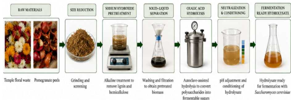
Fig. 3. Process of pretreatment and hydrolysis for bioethanol generation from mixed biomass
