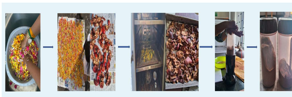
Fig. 1. Experimental workflow for bioethanol production from mixed temple floral waste and pomegranate peel
