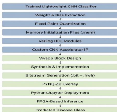
Fig. 4. FPGA deployment workflow for the proposed Lightweight Custom CNN classifier.
