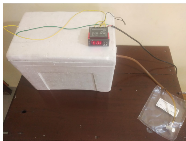
Fig. 9. Dark fermentation setup with gas collection bag (35–37 °C)
