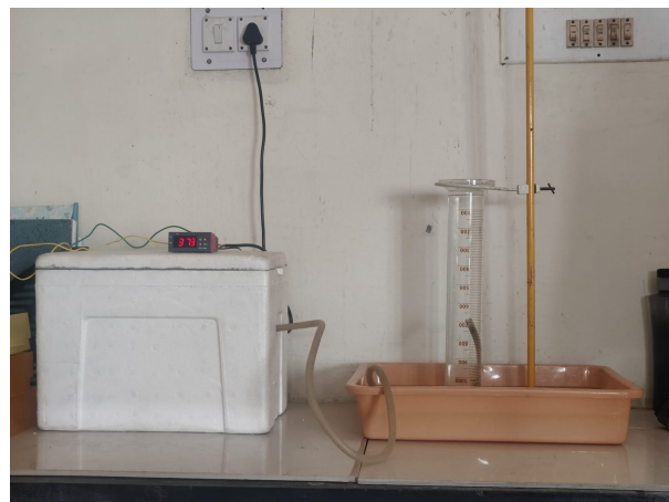
Fig. 8. Dark fermentation setup with water displacement method
