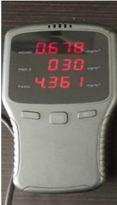
Fig.3 A semiconductor-laser-based air detector to measure PM 2.5 , TVOCs, and formaldehyde
