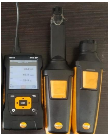
Fig.2 Testo 440 multifunction IAQ meter to record CO, CO 2 , humidity, temperature
