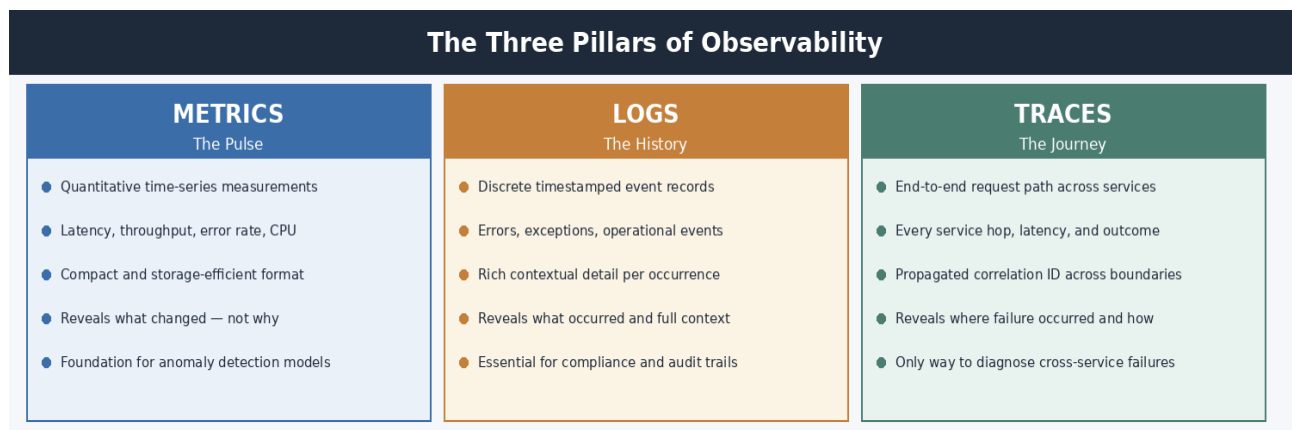
Figure 3 — The Three Pillars of Observability: Metrics, Logs, and Traces each reveal different windows into system behaviour
